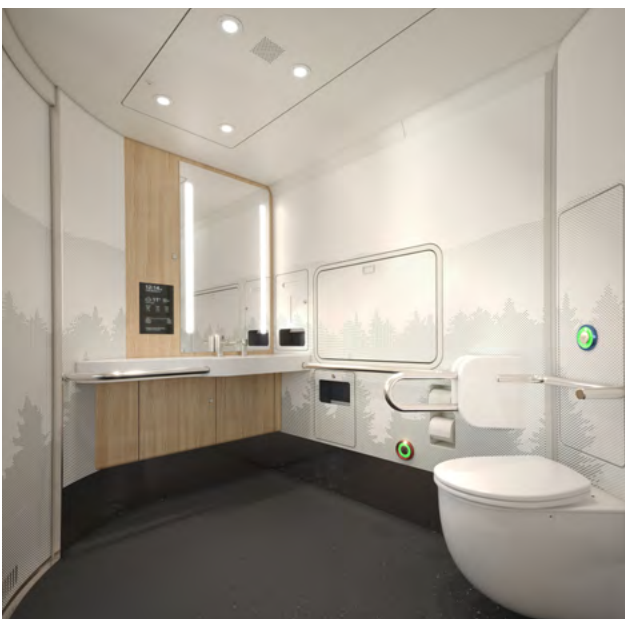
Wheelchair-accessible lavatory designed for the VIA Rail Canada New Corridor fleet
